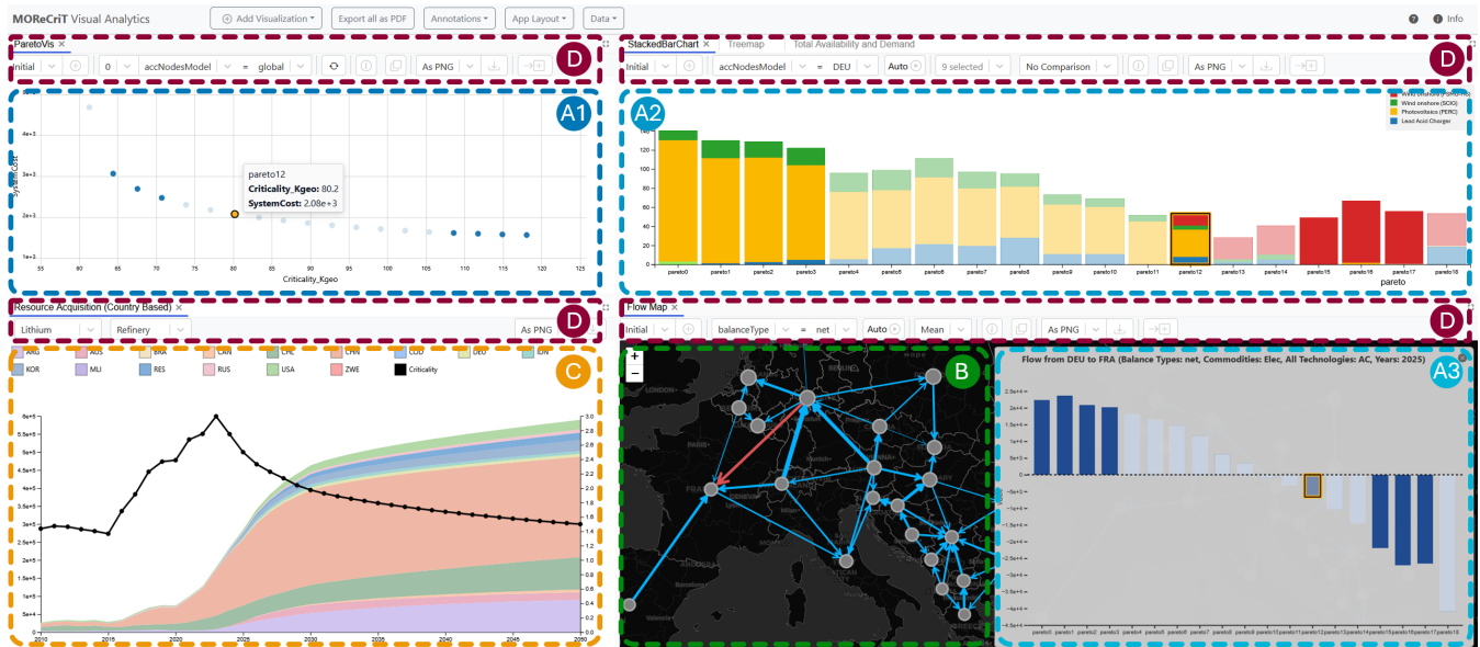
Figure 1: Overview of MORECriT. The Pareto front scatterplot A1 provides the primary entry point for trade-off exploration, here with a selected solution (pareto12, highlighted in orange) that mediates between the cost- and criticality-extreme ends of the front selected via the LinkGroup feature. This selection propagates to the stacked bar chart A2 , which reveals the underlying technology build-outs per country across all Pareto solutions, and to the bar chart overlay on the map A3 , which quantifies energy flows between two countries as selected on the map visualization B . The stacked area chart C integrates input data by showing lithium refinery volumes broken down by supplying country alongside an aggregated criticality line, which spikes when refining is concentrated among a few countries. Each visualization panel provides dedicated adaptation and fixed interaction options D , including export and data selection options.
